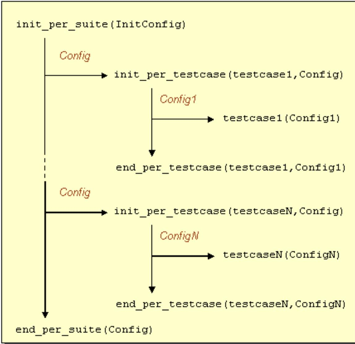
Figure 3.2: Configuration Data Flow in a Suite
